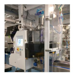
The **tna** robag <sup>FX</sup> 3ci was also customised with product-in-seal-detection (PISD) software that monitors product in the seal and jaw area. If seal integrity is compromised, the system immediately alerts the operator so that bags can be guickly removed from the line for further inspection. That way Pipers Crips is able to ensure that each bag meets the highest quality standards while keeping waste to an absolute minimum.
