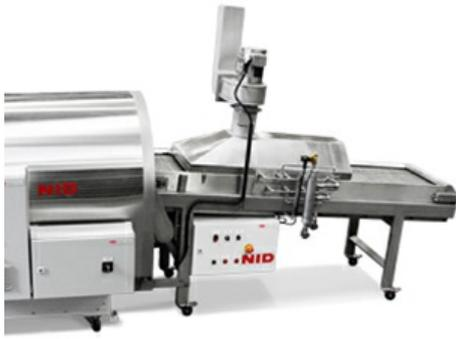
The NID supra-fin<sup>SC</sup> 3 uses a continuous process to cover starch moulded jelly and gum-based confectionery with an even coating of sugar granules, creating a sweeter taste and frosting effect for your product. The NID supra-fin<sup>SC</sup> 3 consists of a steaming conveyor and sugar sanding drum that can be fully integrated into a mogul confectionery processing line, matching production up to 3600 kg/hr (7936 lbs/hr)
