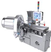
Accurate and consistent coverage and flavour dispersion with directly controlled oil spray and flow of seasoning powder into the drum
