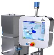
Programme parameters are stored as recipes and easily adjusted via a touch screen
