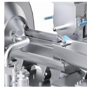
Multiple feed pans for accurate mass flow control of product into the flavour drum
