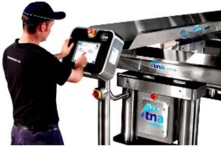
**tna roflo<sup>HM</sup> 3** is the ultimate horizontal conveying system that moves product via a slow forward horizontal motion followed by a fast return horizontal motion. Due to no vertical element, the **tna roflo<sup>HM</sup> 3** minimises flavor fall off and ensures zero flavour build up in the pan.
