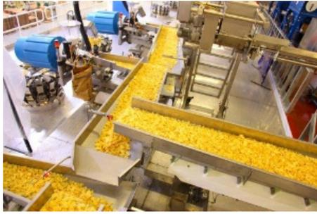
**tna roflo<sup>®</sup> VM 3** is the ultimate vertical conveying system that moves product via vibratory motion. Due to both the horizontal and vertical transportation method, the **tna roflo<sup>®</sup> VM 3** is well suited to even out product highs and lows, and offers the most efficient method for in-line storage.
