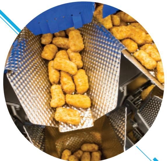
Helping to realise further performance benefits, the packing system was fitted with the **tna** intelli-weigh® omega 314 multi-head weigher. With capabilities for a 2,200 kg per hour in-feed to the packaging system, it was imperative any upstream equipment could keep up with the fast speed of the bagger. The integration of the **tna** intelli-weigh® omega 314 allowed for high speed weighing with superior precision.
