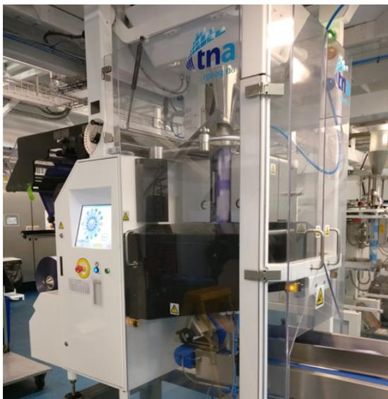
The **tna** robag<sup>FX</sup> 3ci was also customised with product-in-seal-detection (PISD) software that monitors product in the seal and jaw area. If seal integrity is compromised, the system immediately alerts the operator so that bags can be quickly removed from the line for further inspection. That way Pipers Crisps is able to ensure that each bag meets the highest quality standards while keeping waste to an absolute minimum.
